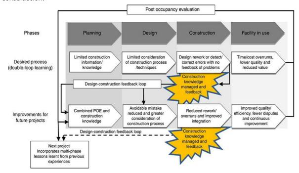
Figure 1. Desired double-loop learning through a design-construction feedback loop (Henderson et al. 2013)
