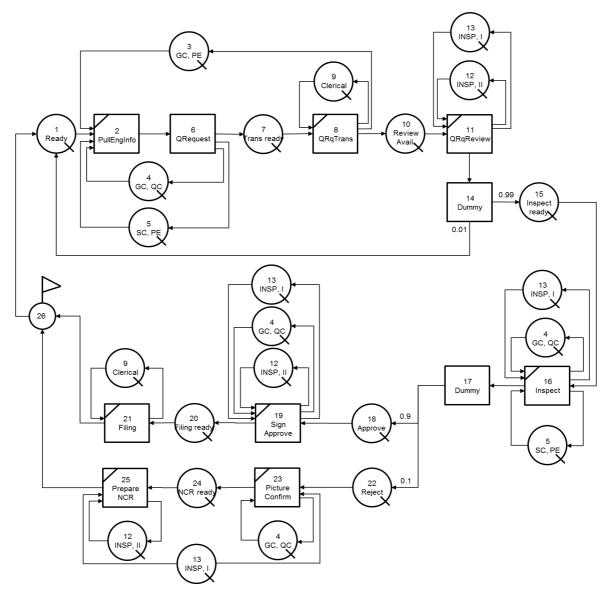
Figure 3: Process model for pipe installation inspection by using CYCLONE simulation
